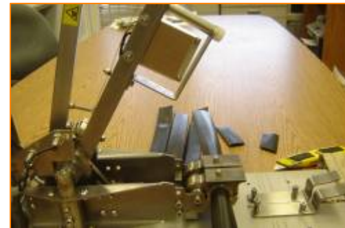
Welding the splice
