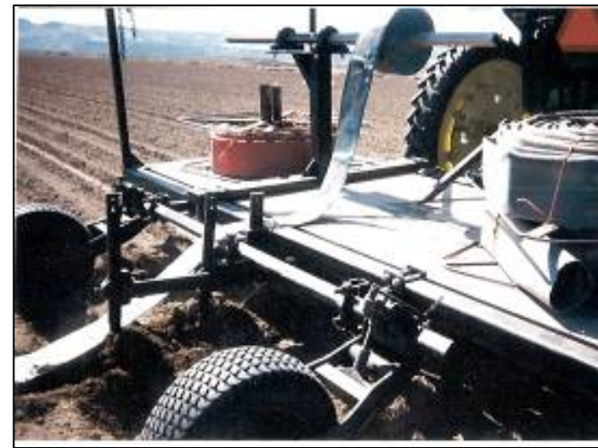
Lay Flat Installation machine
