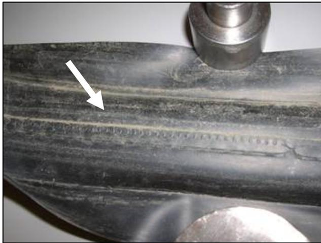
**Figure 11. Plugged inlets to the emitter path**
