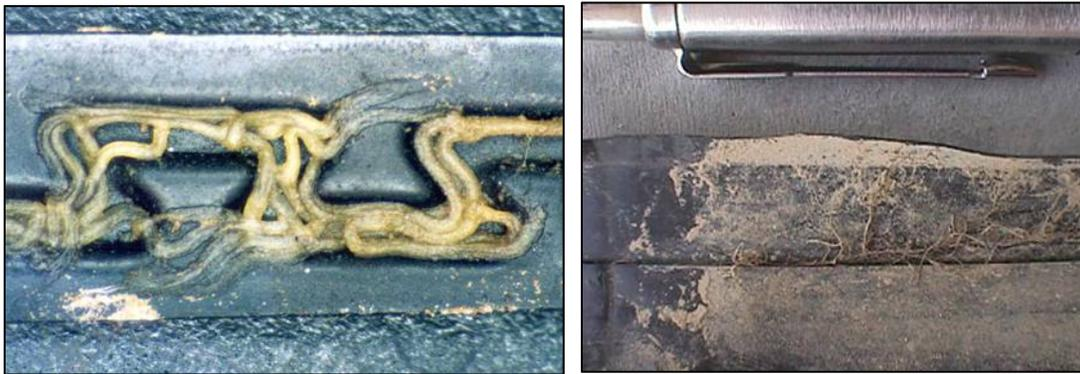
Figure 9. Examples of root intrusion
