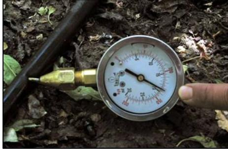
**Figure 1. 30 psi oil-filled pressure gauge with pitot tube stuck into tape**
