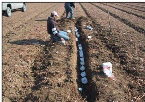
**Figure 3. Plastic containers lined up in preparation for flow measurement of individual emitters. Notice the pressure gauge in the foreground.**
