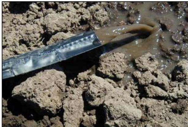
**Figure 12. Dirty flush water. This is an indication of impending plugging problems**
